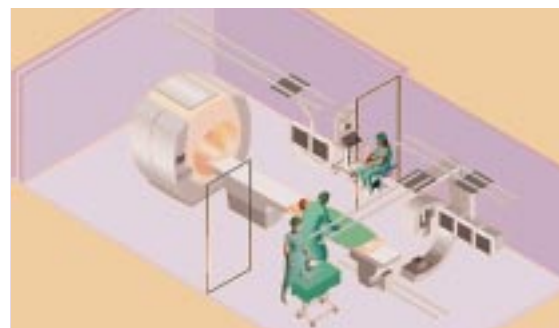
Fig. 1a. The combined MRI/X-ray angio suite. The diagram illustrates the 'two-room' concept: the MR and angio bays are separated by a sliding door allowing them to be used independently or together. For mixed modality imaging, the tabletop carrying the patient can be slid in-line through the open door between the two rooms of the suite.
